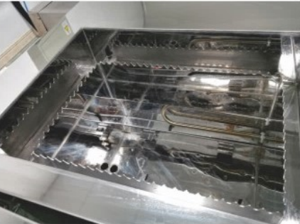
锯齿溢流式超声波清洗槽 sawtooth overflow tank
